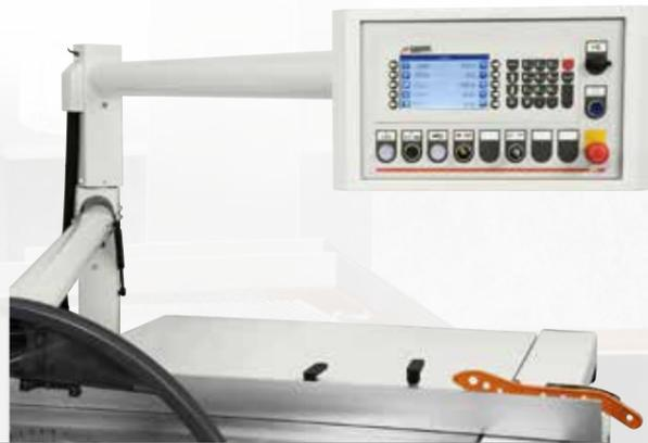
Overhead control panel, available on request only for Xenia 60 A and Xenia 70 A.
