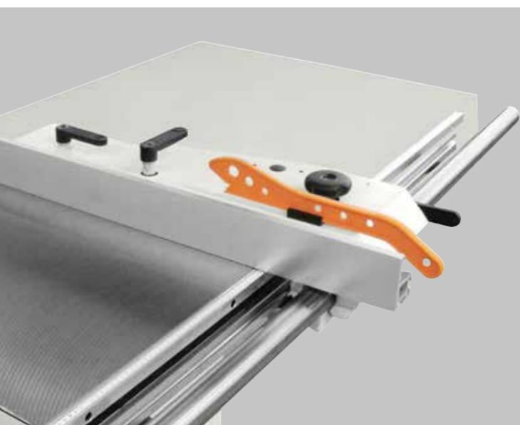
Heavy duty rip fence with micro adjustment through rack & pinion, and fast lock through eccentric. The fence slides over a rectified round steel bar and is fully excludable under the table. The fence can be easily flipped over 90° to enable safe ripping of thin and narrow workpieces.
